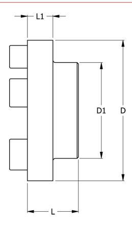
D = 58 D1 = 40 L = 20 L1 = 8 Max bore = 24 Torque (N m) = 19
